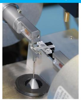
The Dia-Stron FTT950 Fibre Torsion System is specifically designed to measure the torsional properties of single fibres & filaments
