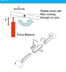
$Torque = Force(F) \times Lever Arm Length(L)$
