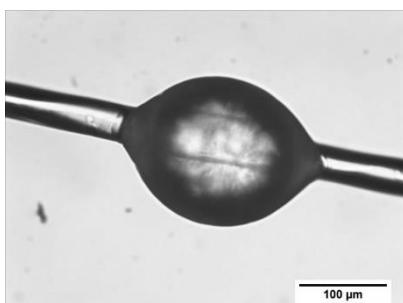
Above: Lyocell fiber with polypropylene droplet
