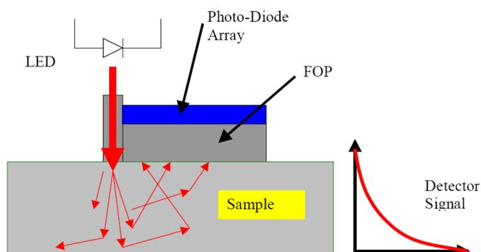
The hand-held probe consists of an RGB led light source and a fibre optic faceplate to transit backscattered light to a NMOS photodiode array. The captured signal is digitised by a microprocessor and the data corrected for background lighting conditions.
