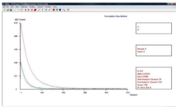
The results are transferred by a USB link to the MApp software for data collection, display and analysis.
