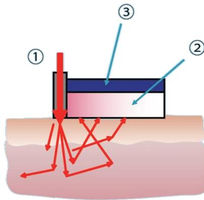
The key feature is that only internally scattered light is collected – not that reflected from the surface as with conventional instruments. The principle of measurement is shown on the schematic diagram above.
